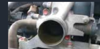
BEFORE (Throttle body condition after 60,000 km)
